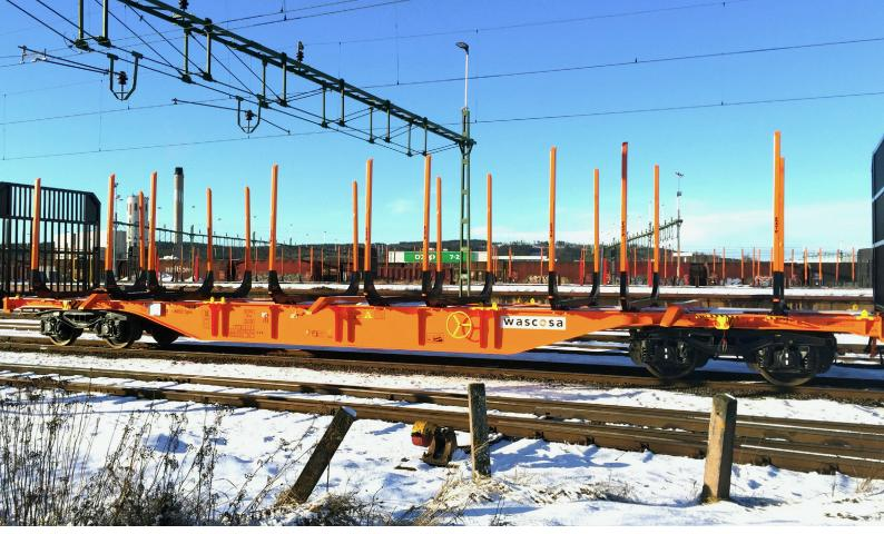
A timber transport wagon was equipped with automatic load weight monitoring at the beginning of the summer. During loading, the weight is recorded in real time and displayed on site and in the web portal. The person responsible for loading can correct overloading or asymmetrical load distribution on site. Photo: PJM
