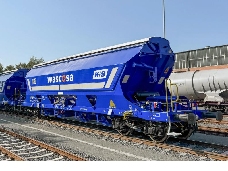
requirements and the need for greater resilience in the K+S transport system were the main reasons for the expansion of the wagon fleet. As well as being robust, the new model offers other convincing advantages: the underframe is 40 cm shorter and the tare weight has been reduced by 1.5 tonnes – this means a higher load volume on the rails, a total loading volume of 78 m<sup>3</sup> and a payload of up to 68 tonnes per wagon.
