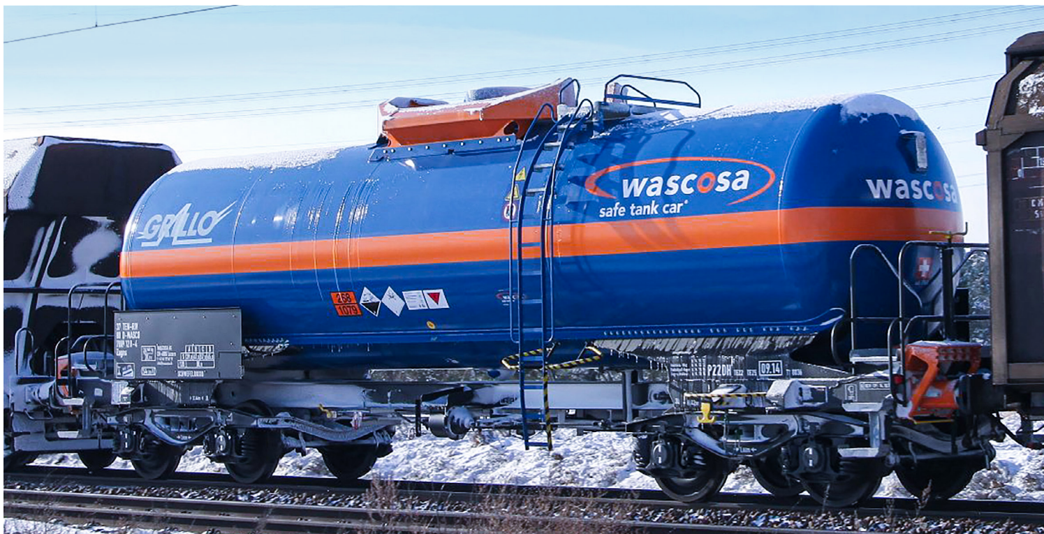
The Wascosa safe tank car®, a product innovation for the transport of chlorine and sulphur dioxide.
