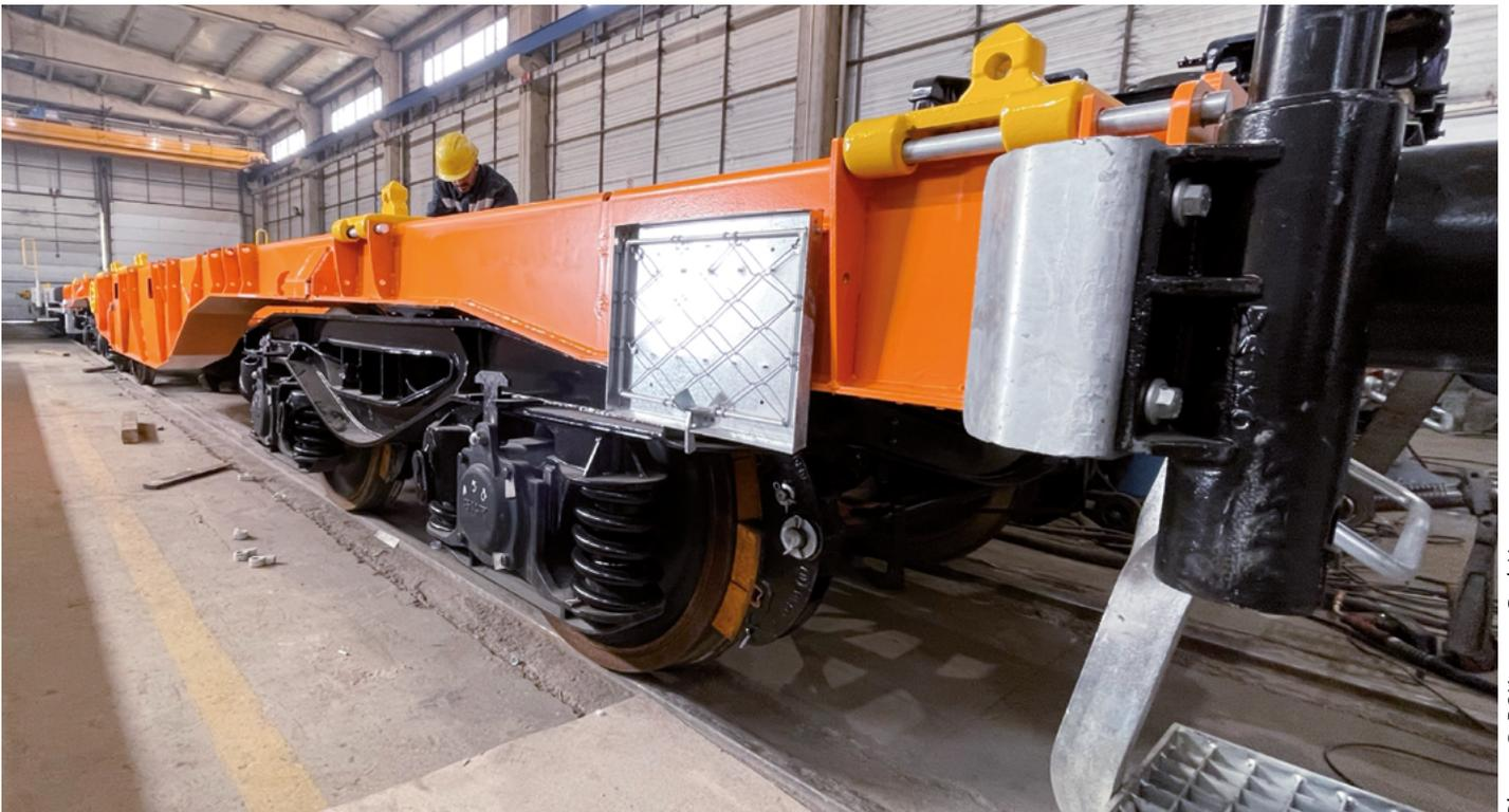
12 months after the start of the project, the finished prototype of the 40-foot carrying wagon was on the rails.
